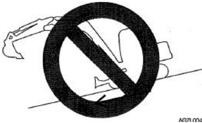
Steep slope when the attachment is lifted
