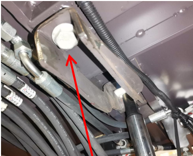
Loose the bolt
